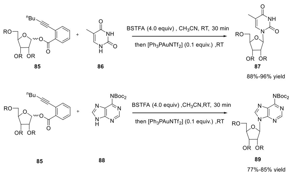
**Figure 15.** Au-catalyzed *N*-glycosylation between glycosyl *ortho*-hexynylbenzoates and nucleobases.
